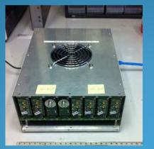
REMOTE READOUT: photodiode & fast ADC
