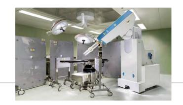
Energy beam: 4-6-8-10 MeV electron beam ; energies according to the tissue thickness measured by ultrasonography of the breast portion to be irradiated
