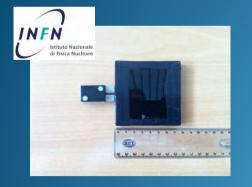
UNDER BEAM: plastic scintillator tile & optical fiber
